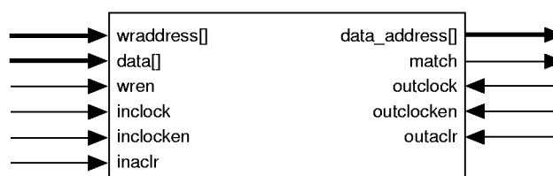
Figure 23. APEX 20KE CAM Block Diagram
